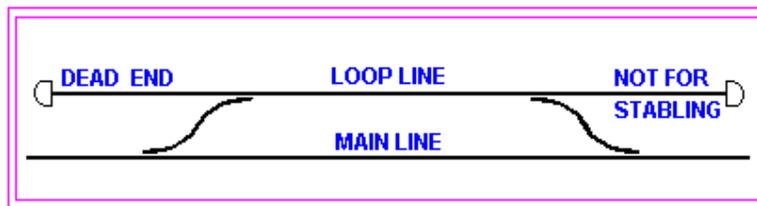
(iii) **Dead End with Trap Points** :- This method is adopted wherever a stabling facility is required.
