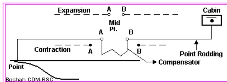
The compensator consists of an obtuse angle crank and an acute angle crank connected by a link. Any movement of the rod on one side due to expansion or contraction is neutralized by an equal and opposite movement on the other side of it.
