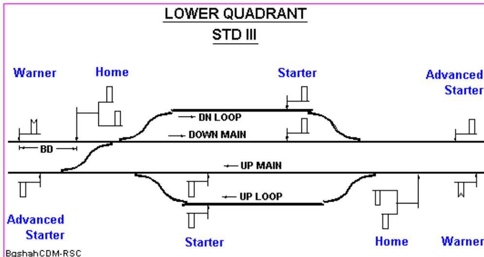
4.4.2 Since Warner is a permissive signal, this does not have a stop aspect and has only two aspects. When the Warner arm is horizontal, it means caution, i.e. the train may be required to stop at Home signal, which is the First stop signal. **Warner lowered to 45-60 degrees means proceed i.e. the train is running through the main line. For run through, via loop line, Warner cannot be lowered. Thus, Warner is lowered only for run through via Main Line.**
