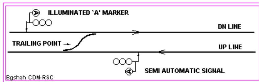
When the points are correctly set for the normal main lines, the signals in both directions work as automatic signals and illuminated A markers are lit up. The rules for passing this signal at 'ON' remains the same as that of an automatic signal. If the points are not correctly set for the normal main lines, the signals in both directions work as manual signals and A marker is extinguished. The driver should get a written memo to pass this signal at 'ON'.
