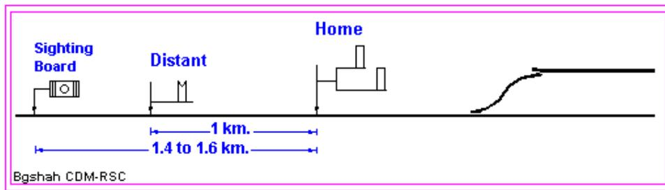
**5.5.2 Passenger Warning Board :-** The Passenger Warning Boards are placed at 1 Km. in case of B.G. and 960m. in case of M.G. in rear of the first stop signal. If the first stop signal is pre-warned by a Warner signal (LQ/A Class) or a Distant signal (in case of MAUQ/MACLS/MLQ), no passenger Warning Board is provided, the permissive signals themselves serve the purpose of Warning Board.
