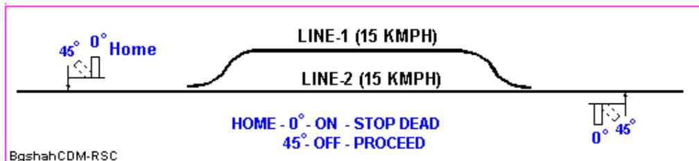
4.1.2 The disadvantage with this arrangement is that there is only one signal protecting any obstruction in the station. If by mistake any driver ignores this signal, there is a possibility of a serious accident. Hence it is necessary to have a second line of defense by adding one more signal in rear of home signal. This signal is called an **Outer signal**.
