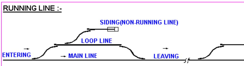
In the above sketch the siding is not a running line, because no train can directly enter or leave or run through the siding.
