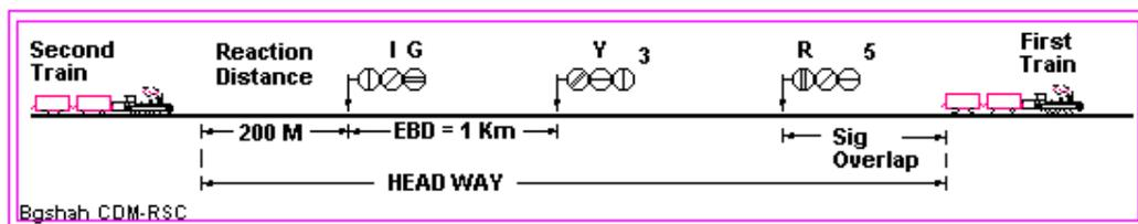
14.5.3 Automatic Block Section with four aspect signals - In case of an automatic section with 4 aspect signals, an automatic signal displays
